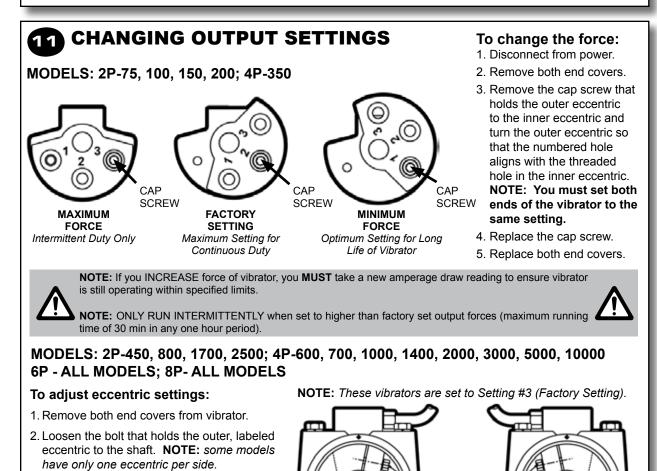
3. Turn the eccentric on the shaft to adjust force output. Align the arrow on the shaft to the desired setting. The higher the number, the greater the force.
