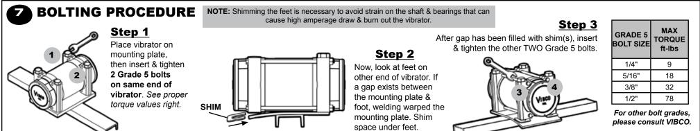
Now put vibrator in place. Make sure it is secured tightly. Retighten bolts after first 10 to 15 minutes of operation and check periodically to maintain proper tightness. Damage to both bin and vibrator can occur if vibrator is not mounted securely. NOTE: no matter how thick the mounting plate, it can still warp during welding, especially if VIBCO's instructions are not followed.
