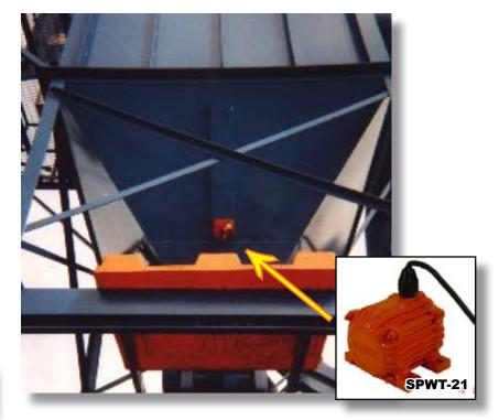
A customer was having problems with dust sticking to sides of bin, all the way down to discharge rotary valve. The bin would have to be cleaned and the product removed from sides of bin. This caused shutdowns in production and was very laborious for employees.
