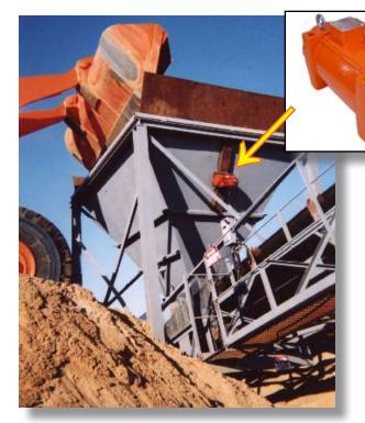
A construction company was having problems with damp sand clumping in their mesh screen on top of their hopper. The sand would clump and production would halt and the mesh screen would have to be cleaned.
