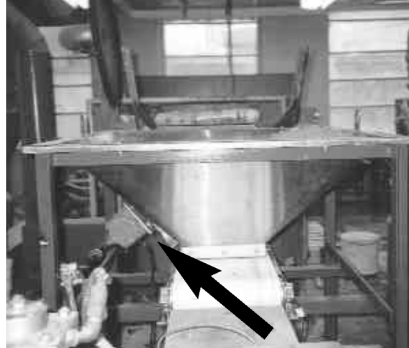
Model 2P-150 on hopper feeding conveyor belt
