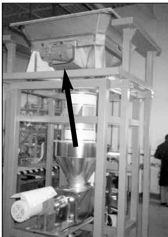
SCR-500 on Box Dumper to prevent hang-ups.
