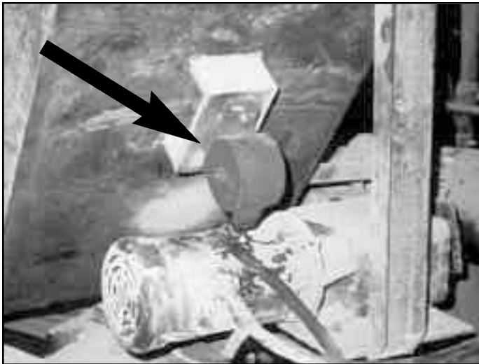
SILENT Turbine mounted to a fly ash chute to keep ash flowing.
