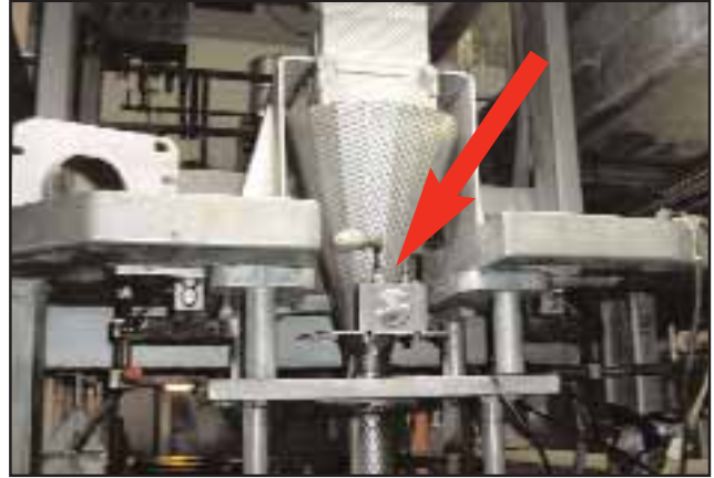
MLTSS-130 STAINLESS STEEL TURBINE VIBRATOR ON TRANSITION CONE FEEDER keeps baby carrots from clogging feeder cone and meets sanitary requirements for food processing application.
