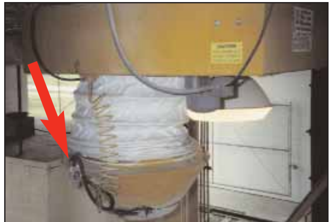
FBS-160 SILENT TURBINE VIBRATOR ON LOADING SPOUT reduced noise levels and increased employee productivity. More installations planned!
