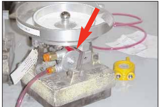
BBS-130 SILENT TURBINE VIBRATOR ON BOWL FEEDER reduced noise to acceptable level and kept product contaminant-free because no lubrication needed.
