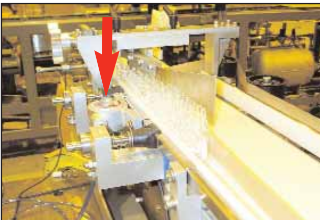
VS-100 SILENT TURBINE VIBRATOR ON BELT FEEDER keeps vaccine bottles in line so they feed through the lane reduction without getting stuck or breaking.
