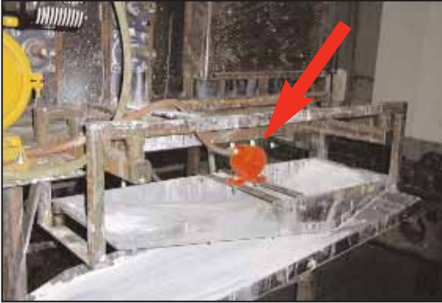
VS-320 SILENT TURBINE VIBRATOR ON PAINT SLURRY reduced surface tension and increased product flow significantly so paint no longer built up on slurry.
